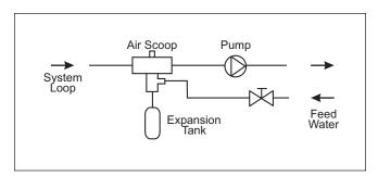
Figure 6B. Typical Plumbing Installations.
